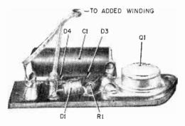
Dry-cell eliminator is about same length as two power transistors. Its thickness is about that of penlight cell and can be fitted into most metal-cased VTVMs.
