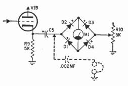
A single earphone, or a set of high-impedance headphones, can be permanently connected to C5 through a small capacitance without upsetting the calibration of the meter.
