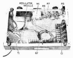
Regulator circuit is made into a module to provide better temperature stabilization but it's not a worry for most experimenters.
