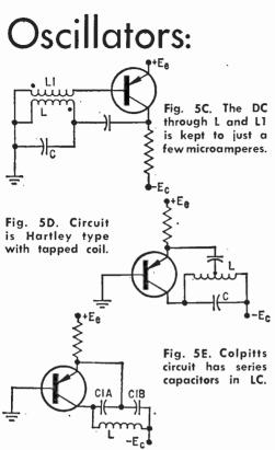
Fig. 5C is basically the same as Fig. 5A except that the tank (LC) circuit is ACcoupled (shunt-fed) to the collector with a capacitor. The current in Fig. 5D can be compared to that in 5B. The autotransformer action of the tank circuit is used as the feedback circuit with capacitor C1 used to block DC between the collector and the emitter. Fig. 5E is similar to 5A and 5D except series capacitors are used, in place of a tapped inductor, to provide the feedback path.
