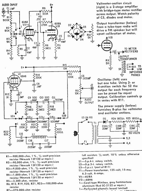
of C5, diodes and meter. **Output transformer (below)** from a tube-type radio will
