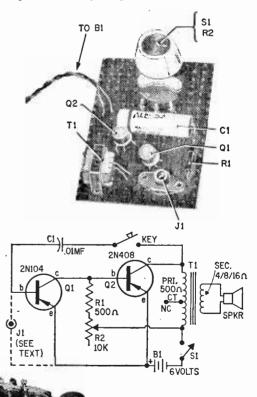
Fig. 6. Code-practice oscillator has standard parts. R2 controls volume. With key open, J1 can be used as an input to amplifier circuit.
