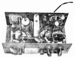
For all-day operation better drill more vent holes in the cover directly over V1 and V2.
