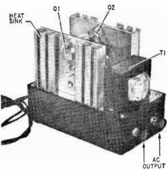
Fig. 8. Any standard inverter transformer can be used for T1-just watch the ratings.
