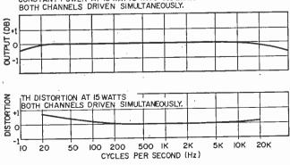
ACOUSTECH XI POWER AMPLIFIER CONSTANT POWER AT 15 WATTS INTO 8 LOAD. BOTH CHANNELS DRIVEN SIMULTANEOUSLY.
