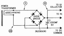
Fig. 4. Bridge rectifier circuit doubles ripple frequency and improves filtering.
