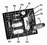
Fig. 7. Broadcaster is a phono oscillator modulated by a high-output phono cartridge. Carbon microphone or mike and preamp are needed for voice broadcasting to AM radio.
