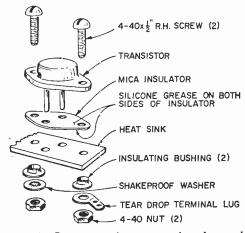
Fig. 3. Power-transistor mounting is much easier on pre-drilled heat sink—otherwise use insulating washer as a drill template.
