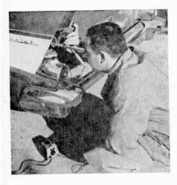
Peering into eyepiece of fiberoptic tube, technician is actually viewing the inside of a generator. Curving tube doesn't bother light waves one bit. They flow like water inside a garden hose.
