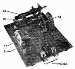
Parts layout is not critical. Just keep lead lengths (wires) between C1, L1 and Q1 reasonably short. RF-bypass or filter (C2) controls average voltage from detector—too high a capacitance will affect treble tones of music —effect will be noticeable with hi-fi phones.
