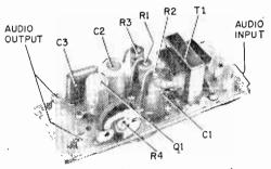
This is just about the most compact layout possible. Transformer T1 is the largest component perforated board. Resistors and capacitors could be wired flat instead.
