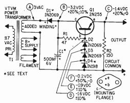
Fig. 1. Hardest part of this circuit is adding winding to existing transformer.
