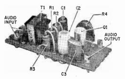
Completed perforated board showing components in place; note spaghetti on the leads.
