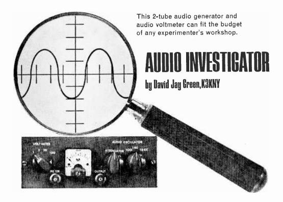
■ Ever wonder which stage in your multistage hi-fi amplifier isn't working, or how much gain it has? Well, with this one unit troubleshooter you can solve these problems. Using the oscillator and voltmeter sections, the gain of amplifiers can be measured. Frequency response can be spot checked—the oscillator section has output at three frequencies; low (100 cps), medium (1 kc), and high (10 kc).
