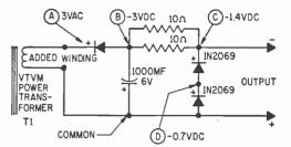
Fig. 5. This simpler circuit doesn't use a series regulator to load—here load is in parallel to the shunt regulator diodes.
