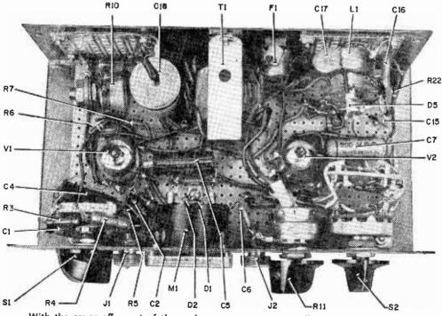
With the cover off, most of the major components are easily located inside unit.
